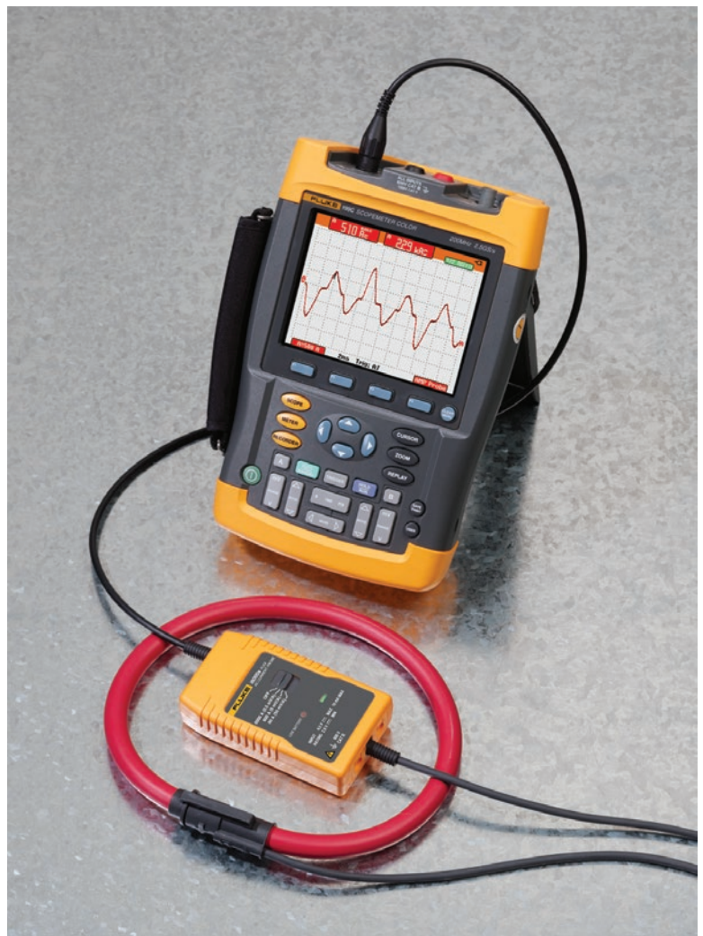
i6000s connected to a Fluke 199C ScopeMeter.
